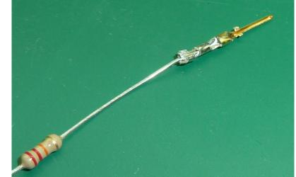
Soldered and the tabs crimped with pliers
