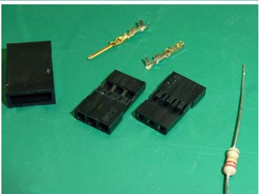
Pin ready for tinning and soldering
